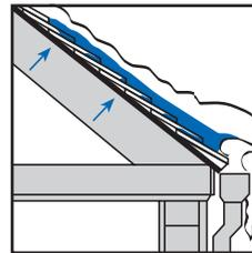
Grace Ice & Water Shield resists this leakage because of the seal around the fasteners, ability to make watertight laps, and the membrane's bond to the deck.
